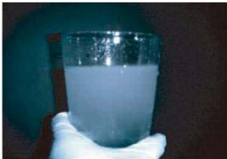
The white bubbles that can be seen here are hydrogen.
